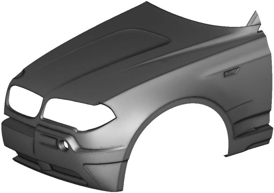
Fig. 5. Curvature representation of the mesh in Fig. 2
